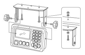
• DASHBOARD MOUNTING (with optional MB-75): For mounting the DS-100 to a dashboard panel.
